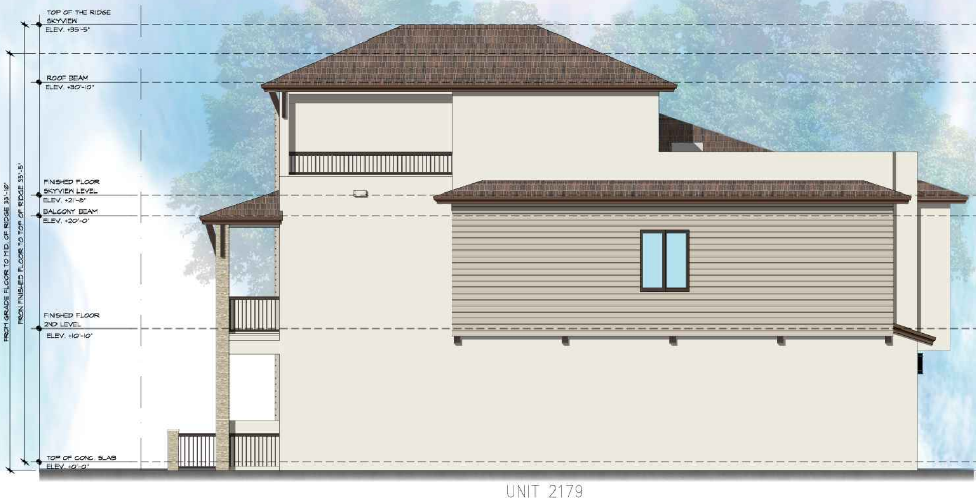
8 UNIT BUILDING LINEAR - RIGHT SIDE ELEVATION SCALE: 1/8" = 1'-0"
