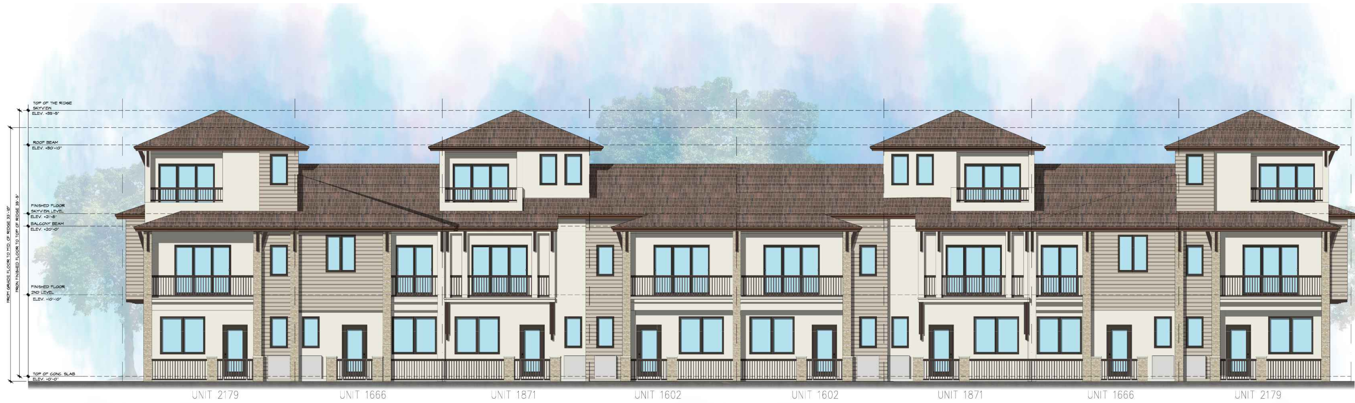
8 UNIT BUILDING LINEAR - FRONT ELEVATION SCALE: 1/8" = 1'-0"
